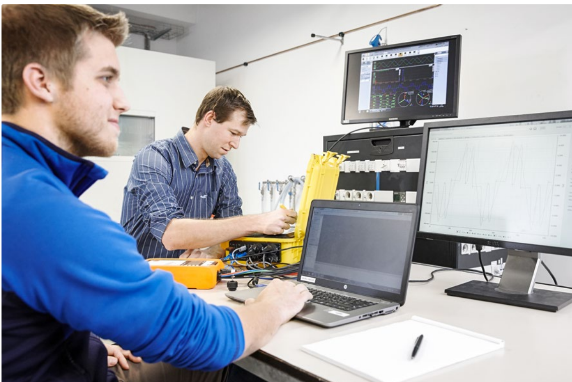
The power quality simulator is used to analyse the sensitivity of small devices to network disturbances, and their effects on the power grid.
