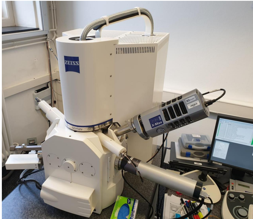
Scanning Electron Microscope (SEM) used for the microstructure analysis
