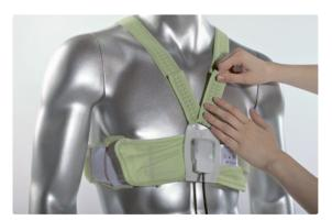
In collaboration with Swisstom AG, BFH has developed a device that optimizes the parameters for artificial respiration. The EIT belt, created by a student Andreas Waldmann, helped pave his way into the professional world. Using Electrical Impedance Tomography, an innovation was started that was transformed into a successful product by our industrial partner.
