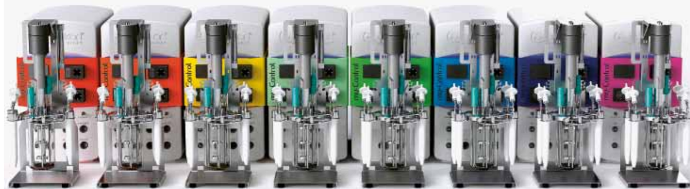
Set of miniBioreactors and corresponding myControls for parallel cultivation experiments. Photo: Applikon Biotechnology BV, Delft
