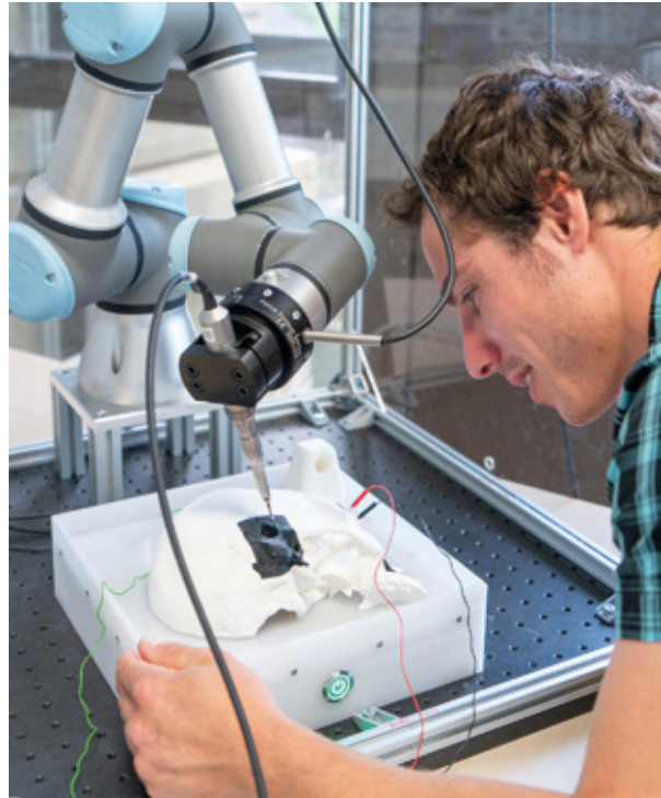
Drilling in a custom-made phantom with nerve monitoring.
