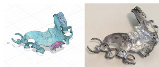
Fig2: 3D-CAD Model of dental prosthesis (left), Additively manufactured part after twelve PEP-Jet polishing processes (right)
