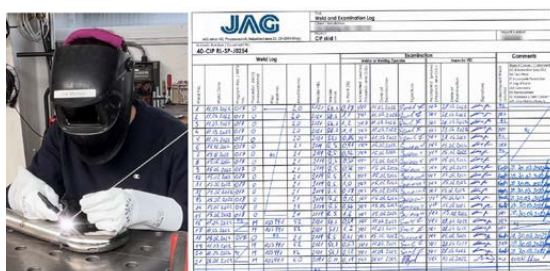
Figure 1: Welder at work and Weld Log in paper form with all the welding data and signatures of the welders and inspectors.
