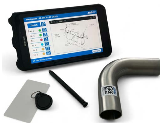
Figure 2: Prototype application with NFC tags and Matrix code on a pipe, that will be welded into a pharmaceutical plant.
